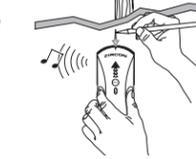
Without releasing the Power button, continue scanning beyond the marked spot until the red EDGE light turns off. Slide unit in reverse direction to locate other edge of stud.
