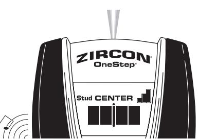
In cases of deeper studs (or thicker walls) two bars will show on the Signal Strength Indicator and only the SpotLite® Pointing System and four middle bars will illuminate. If you still can't locate a stud, try DEEPSAN® mode.
