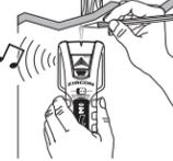
Without releasing Power button, continue scanning beyond marked spot until some segments of the arrow turn off. Slide unit in reverse direction to locate other edge of stud.
